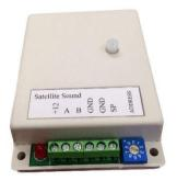
This tiny module 9cm \* 7cm enables you to produce any of the Bestlite alert sounds and levels into a speaker at any location and operates from the standard Bestlite RS485 buss.
