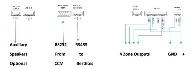
The zone inputs on the CPI are not polarity conscious. Connect one side to the 24V + supply and the other side to the negatively switched zone outputs on the NIM. The 24V supply to both NIM and CPI must be common or at least have a common ground.
